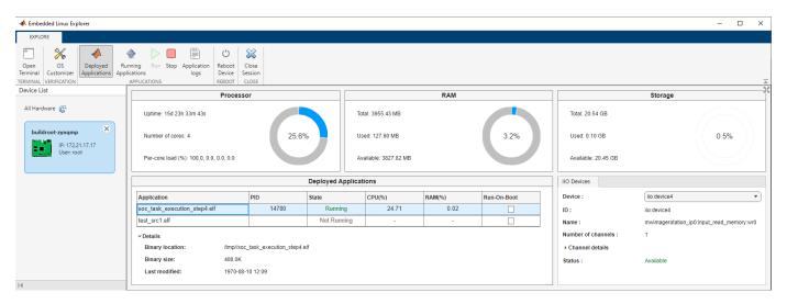
To run the application every time the board reboots, select the row for the model in the **Deployed Applications** table, and select **Run-On-Boot**.
