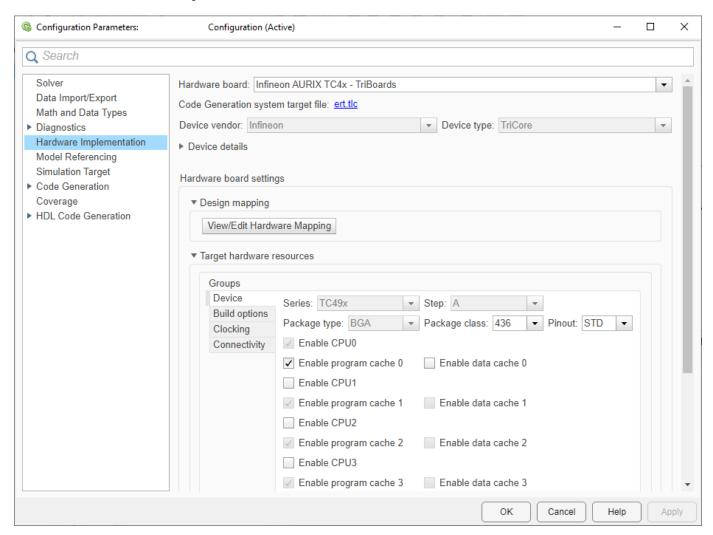
Configure hardware board to run Simulink models.
