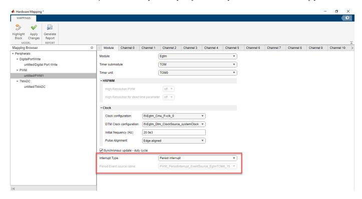
Selecting this option also enables the read-only parameter **Period Event source name**, which provides information on the source of the period interrupt. The source depends on **Module**, **Timer submodule**, and **Timer unit** parameters. You can map the name in the tasks (CPU1).
